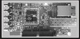
There are max. 4pcs (supporting LAN3-10) autonomous PTP/IEEE1588 grandmaster cards inside NTS-5000. They are all 100% isolated (no TCP/IP communication). Server provides Time Domain to all 4 cards via internal SyncBUS.
