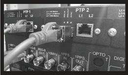
Autonomous cards operate in high accuracy Time Domain. PTPT/IEEE1588 card #1 can be set to operate SLAVE mode. All 1-4 cards support PTP GRANDMASTER with profiles: ENERGY, TELECOM, ENTERPRISE and FINANCIAL.
